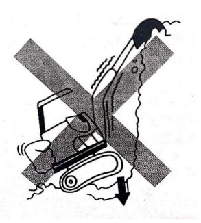
4. It is forbidden to use driving power for work. (Insert the bucket into the ground to drive, etc.)
